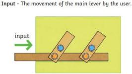
Output - The movement that is made by the smaller levers.
